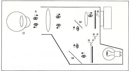
Fig 1.—Circular polarizer. Retarder transforms linearly polarized light into two orthogonal components and retards one of these components by phase angle of 90°, one quarter wavelength.
